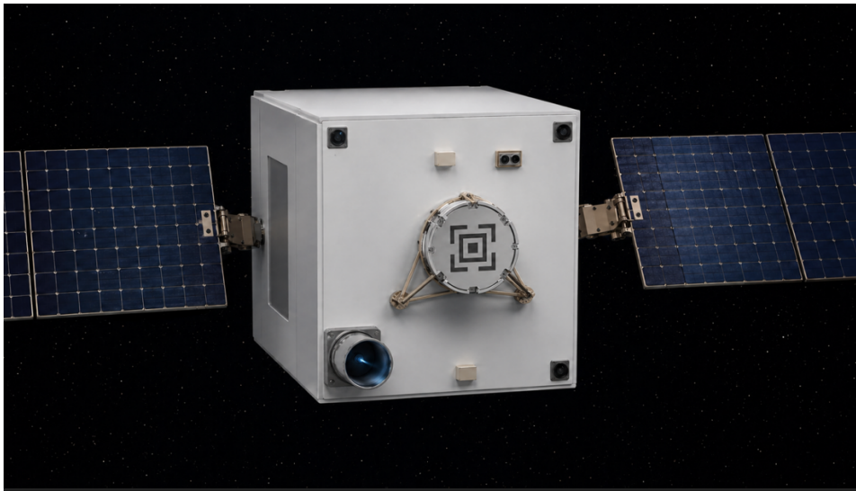
Figure 2 Illustrative render of the docking plate integrated on a synthetic SDA-class reference bus. The plate is mounted at the geometric center of the anti-velocity face with its Y-axis aligned with the bus center of gravity. The gimbaled Hall thruster is mounted off-center on the same face. Bus geometry is representative, not a specific flight design.
